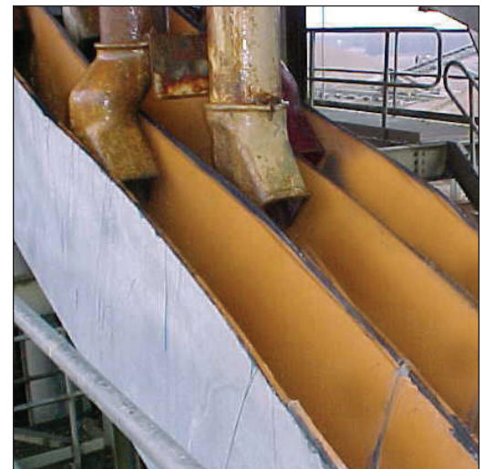
Wash flumes in a sand and gravel processing facility.
